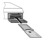
Common Interface (CI) is an interface for conditional access modules. The front of the digital receiver has two common interface slots.
